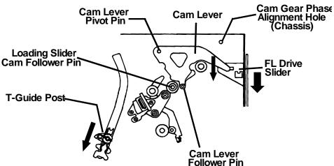
Before installing the Cam Gear its very important that the Cam Lever and the Loading Slider cam follower pins be positioned properly. This is important because the cam groove follower pins must fall into their proper grooves on the underside of the Cam Gear.
