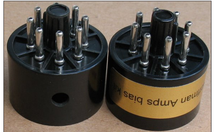
The tube bases with the wire hole already drilled and a nice gold sticker
