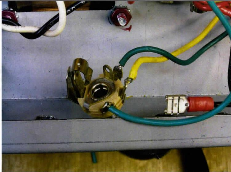
The aux jack switches the load to 4 ohms when you plug in a second speaker. Attach the yellow and green wires from the TO22/TO26 as shown. Take care with the attached green wire with the push-on connector. Moving it back and forth too much will fatigue the wire and break it. **The center lug (ground) is left empty.** The jack is grounded through the chassis.
