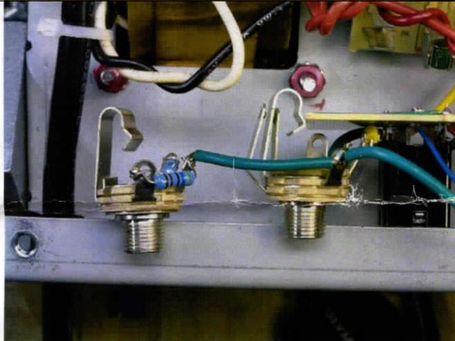
If you ordered the line out jack, it is attached by a short green wire. Don't over-handle or over-bend the wires.
