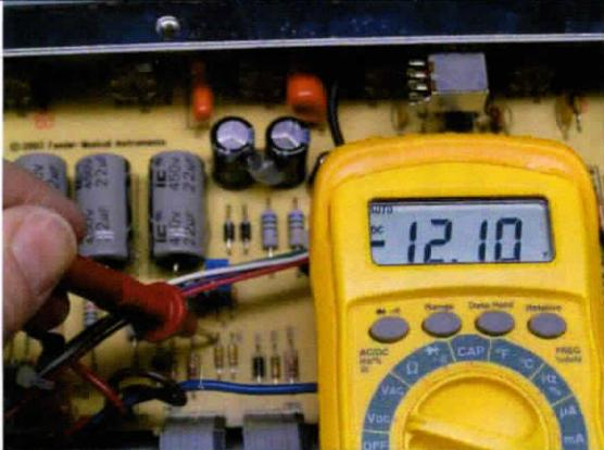
The trimpot has been shipped to you set at the midpoint. If you didn't turn it, you should get a reading of roughly -12V to -13V between the top of either R31 or R32 and ground. This is a safe bias voltage that won't red-plate your tubes.
