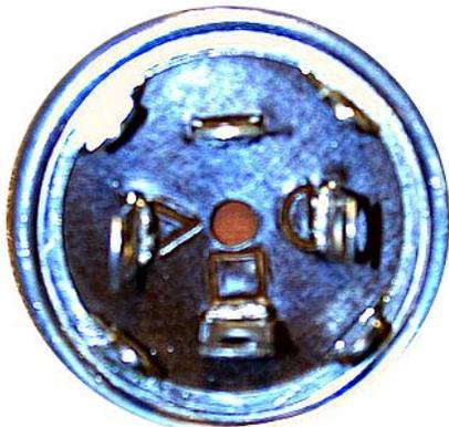
**Important:** Mark each wire going to the old can capacitor with a piece of tape labeled with the symbol for the terminal to which it attaches. Also make a note of the orientation of the old capacitor (which side the symbol is facing, for example). Install the new capacitor in the same orientation, so that the wires will have sufficient length to reach the proper terminals. Solder the wires to the terminals as per their tape labels.
